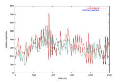
Figure 4: AVO of a strong reflector event at 1.8 s extracted in the common-image gather for CMP no. 560 after true-amplitude prestack time migration with minimum aperture (dashed line) and conventional aperture (solid line).
