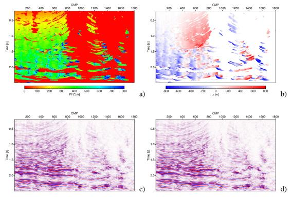
Figure 2: a) Size of the projected first ZO Fresnel zone estimated from the CRS attributes. Only locations with identified stationary points have been considered. b) Horizontal distance between operator apex and stationary point estimated from the CRS attributes. The second row displays the result of the Kirchhoff poststack time migration with c) conventional user-defined aperture and d) with minimum aperture.
