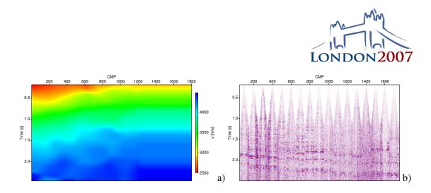
Figure 1: a) Smoothed time migration velocity model determined from the CRS wavefield attributes. b) Several common-image gathers extracted from the conventional time migration prestack data. The maximum offset is 3 km.
