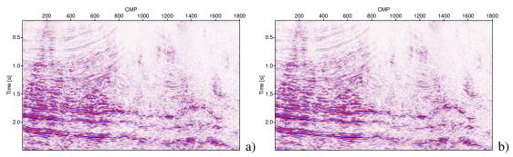
Figure 3: Result of the Kirchhoff prestack time migration with a) conventional user-defined aperture and b) with minimum aperture.
