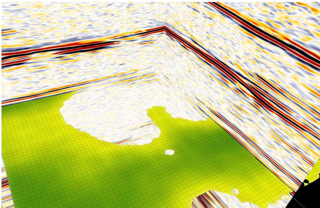
Figure 3: Detailed view of a gap in the tracked reflection event. The gaps are due to areas where no valid continuations were found. The color coding has the same meaning as in Figure 2.
