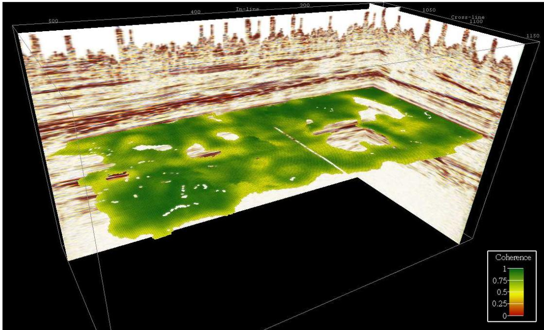
Figure 2: Automatically tracked reflection event. The colors on the surface indicate the respective coherence values. The inline and crossline sections are taken from the CRS stack volume.
