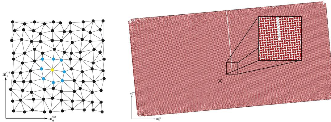
Figure 1: Left: after Delaunay triangulation the nearest neighboring traces (depicted in blue) to an arbitrary central trace (yellow) are given by all the traces that share a triangle with it. Right: Delaunay triangulation of the trace locations (red dots). As can be seen, the distribution of the traces is irregular in the midpoint plane. The cross indicates the starting trace used for the tracking.
